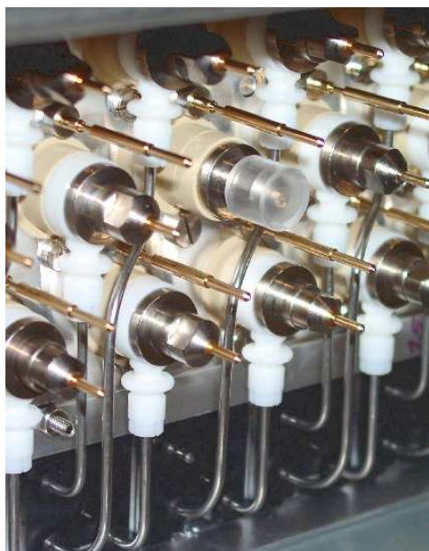
Figure 1: Disconnected tube. The pin of the signal cap is removed and the cap covered with a plexiglas cover which is 1 mm thick and fits without touching the hedgehog card. The gas connection at the triplet is sealed with a stainless steel bolt.
