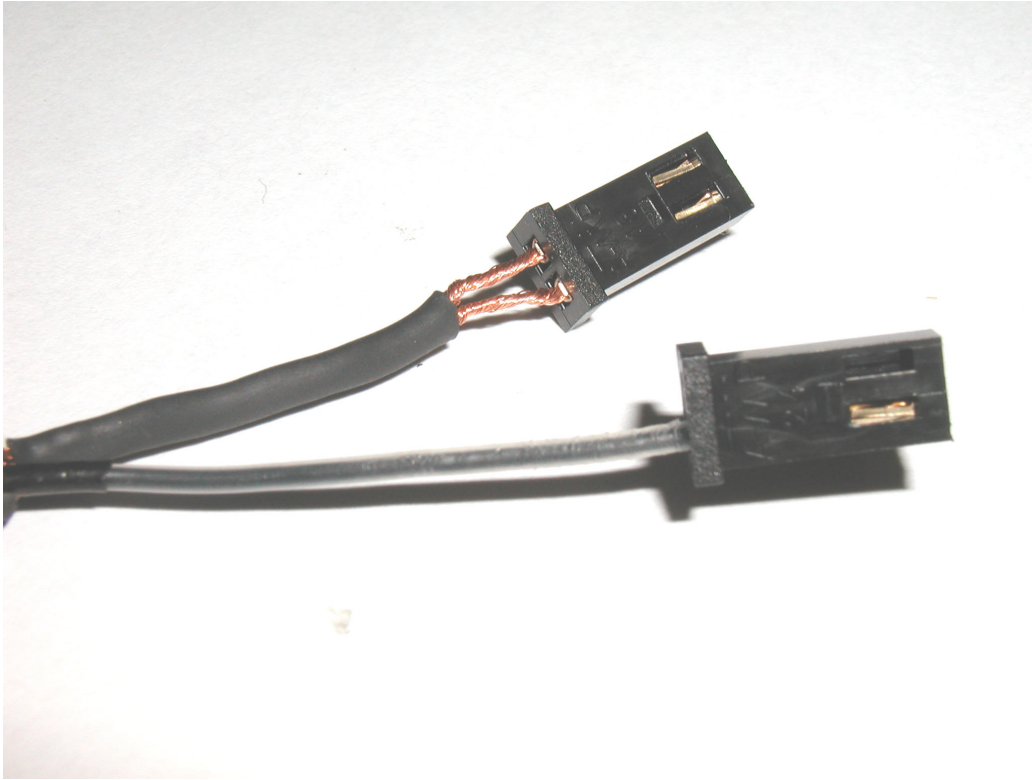
Fig. 6 – AMP receptacles inserted on contacts
